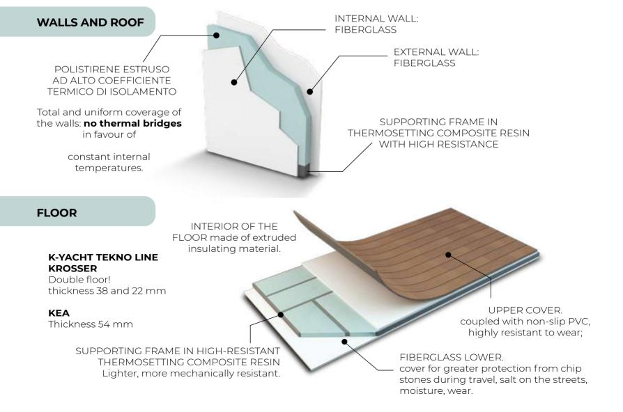
The thicknesses and materials selected for the construction of Mobilvetta floors ensure insulation from below, mechanical resistance and a stable guide on any road surface.
