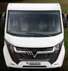
The A pillars feature a reduced thickness to facilitate driver visibility and control over the overall dimensions and movements of the motorhome.
