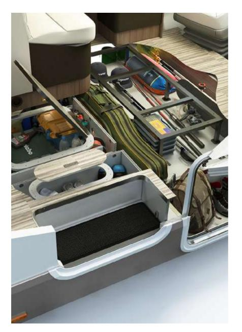
**Lower floor thickness** 38 mm: greater thermal insulation from the outside and greater protection against noise from the underside of the vehicle
